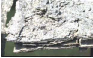
Figure 5. Exfoliation of an Aluminum Alloy in a Marine Environment[2].
