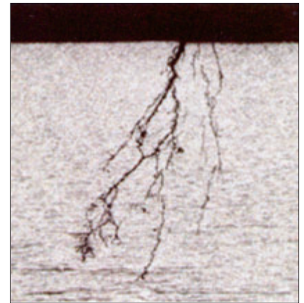
Figure 9. Stress Corrosion Cracking (50X Magnification) in 304L Stainless Steel Pipeline (Photo Courtesy of Corrosion Testing Laboratories, Inc.)[1].
