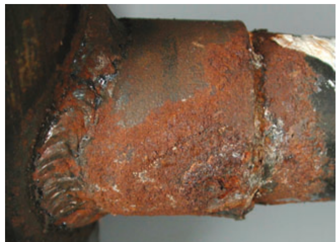
Figure 1. Uniform Corrosion on Iron Piping in a Fire Sprinkler System Caused by Leaks in the Threaded Joints. (Photos Courtesy of Corrosion Testing Laboratories, Inc.)[1].
