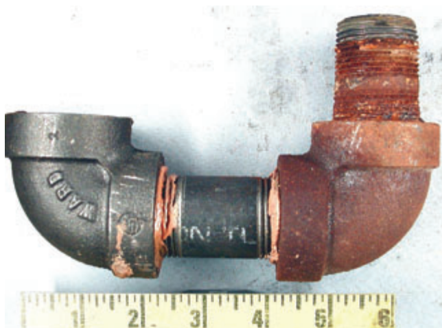
Figure 1. Uniform Corrosion on Iron Piping in a Fire Sprinkler System Caused by Leaks in the Threaded Joints. (Photos Courtesy of Corrosion Testing Laboratories, Inc.)[1].
