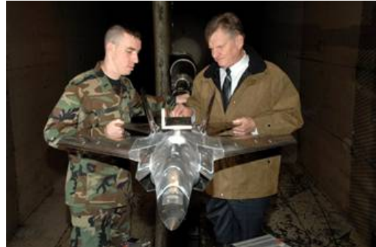
First Lt. Ezra Caplan and Charlie Smith examine a 12-percent scale model of the Navy variant of the F-35 Lightning II joint strike fighter during a break in the final pre-production aerodynamics testing done on all F-35 variants at Arnold Engineering Development Center, Arnold Air Force Base, Tenn. Lieutenant Caplan is the AEDC Air Force project manager and Mr. Smith is the Aerospace Testing Alliance senior project engineer. (U.S. Air Force photo/Rick Goodfriend)
