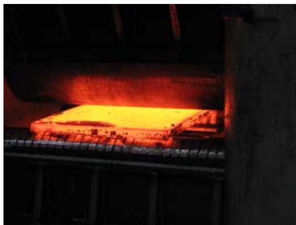
Testing determined parameters for hot forming HSLA-65 and DH-36 plates for CVN 21 and other platforms. (Concurrent Technologies Corporation photo)
