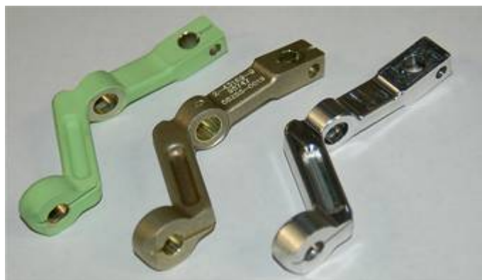
Hill works to replace T-38 aileron levers - Three steps in the manufacturing process of T-38 aileron levers are shown as the part is first custom cut (right); numbered and textured (center); and finally painted green and shipped to the customer. (Air Force photo by Bill Orndorff)
