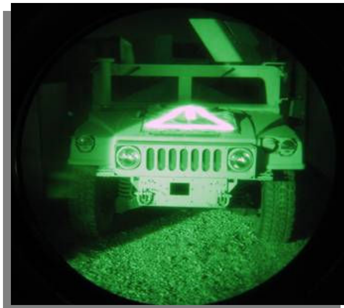
A military vehicle marked with Target Recognition Operator Notification I (small strip in the center) and TRON III is shown through night-vision goggles in January near Bagram Air Base, Afghanistan. The identification technology was developed by Air Force Research Laboratory officials in collaboration with the civilian industry to support joint warfighters. (U.S. Air Force photo)
