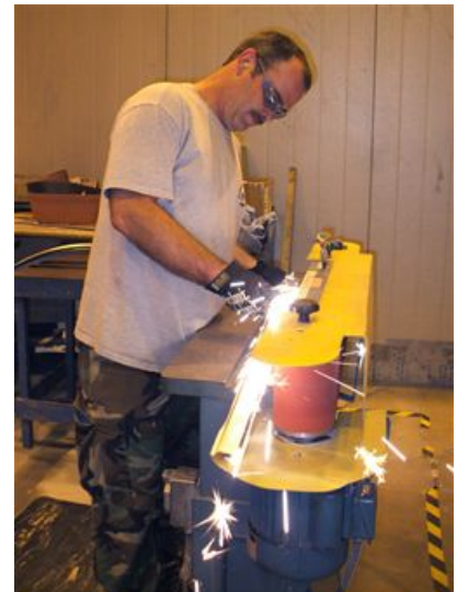
David Stroupe, a sheet metal mechanic, grinds an inconel steel part to the required dimensions for the C-130 IRSS. (Air Force photo by Dave Hoffman)
