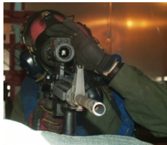
Test Officer Paul Brown adjusts a thermal weapon sight on White Sands Missile Range's Small Arms Range Feb. 7. The structure he is firing from is more than 100 degrees inside and the small space requires that he wear an oxygen mask because of the carbon dioxide being put off by the weapon. (photo by Drew Hamilton)
