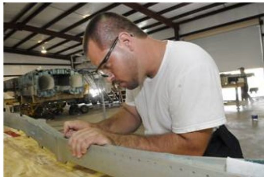
Ben Rogers strips paint and primer off a longeron so it can be sent off for analysis. Rogers is part of a crew that is disassembling an F-15 in an effort to provide maintenance crews more information about the aircraft. (Air Force photo by Sue Sapp)
