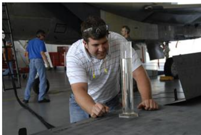
Ryan Mead checks the density of the SJ-8 50/50 blended synthetic fuel before use in two successful F-15 flight tests Aug. 19. Mr. Mead is an F-15 fuels engineer at Warner Robins Air Logistics Center, Robins Air Force Base, Ga. (Air Force photo by Claude Lazarra)
